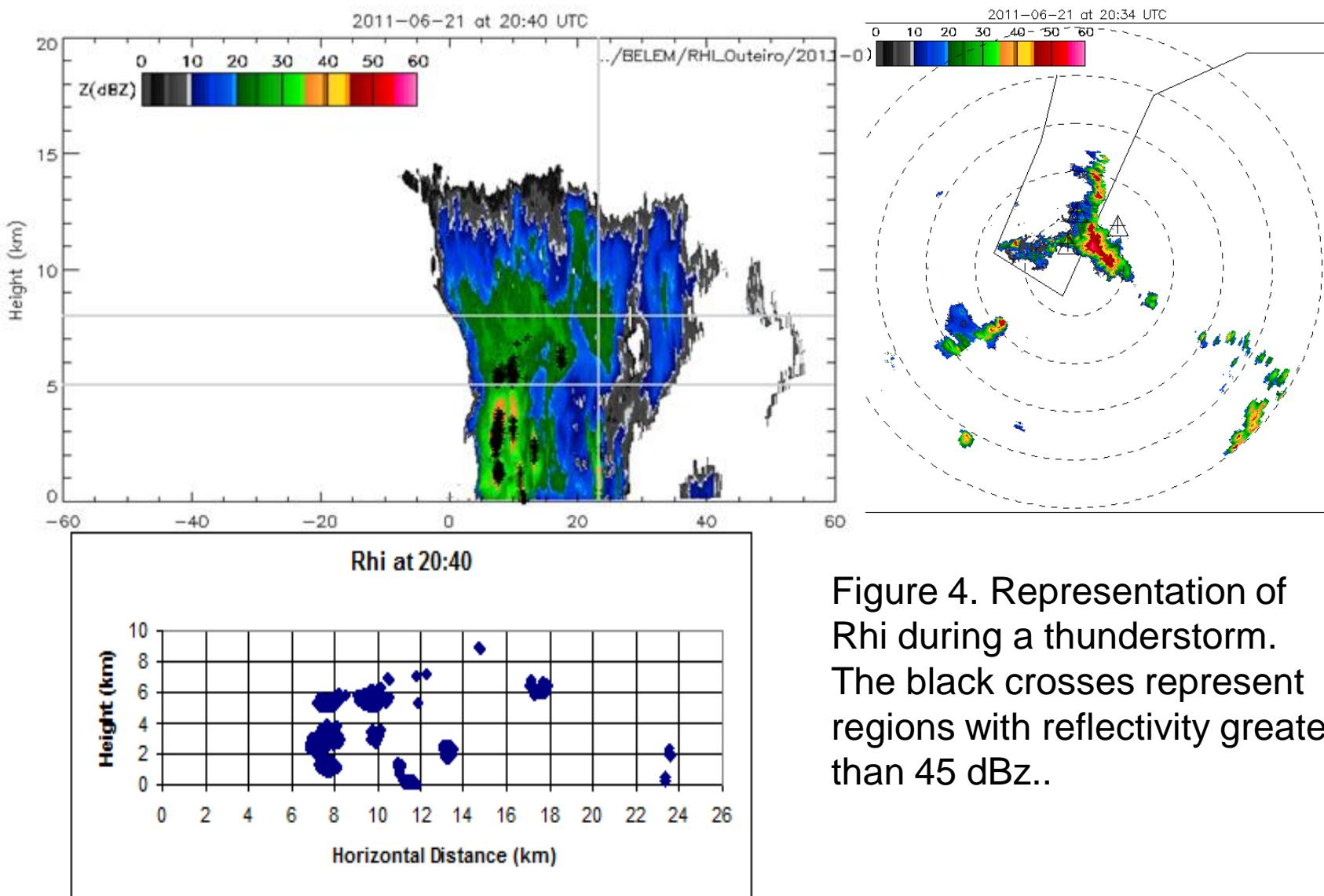
Figure 4. Representation of Rhi during a thunderstorm. The black crosses represent regions with reflectivity greater than 45 dBZ..
