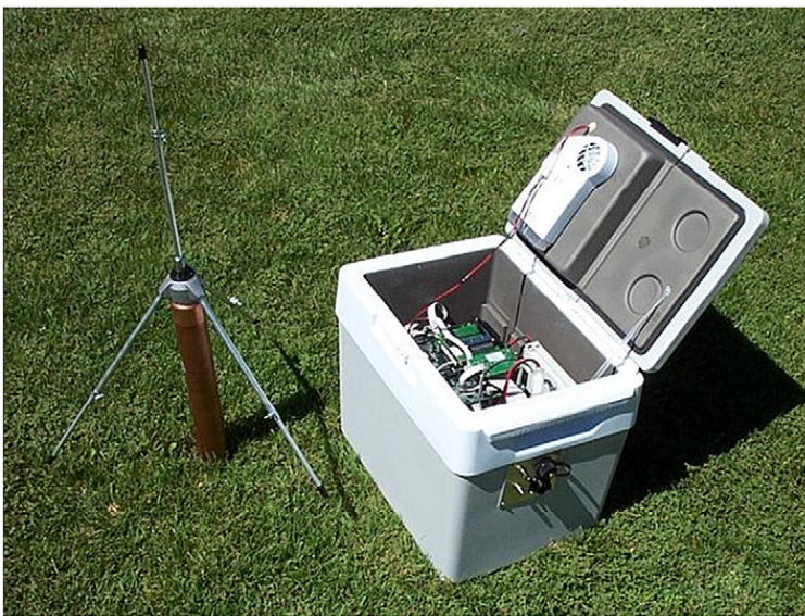
Fig. 9. São Paulo Lightning Mapping Array (SPLMA) station showing the VHF (Channel 8, 162 MHz) ground plane antenna, sensor electronics and computer package (lower left). Plot with horizontal and vertical projections of 1-hour source density for 0100–0200 UTC on 27-Nov-2011 (lower right) encompassing the LIS overpass 0131–0135 UTC and WWLLN observations (above).
